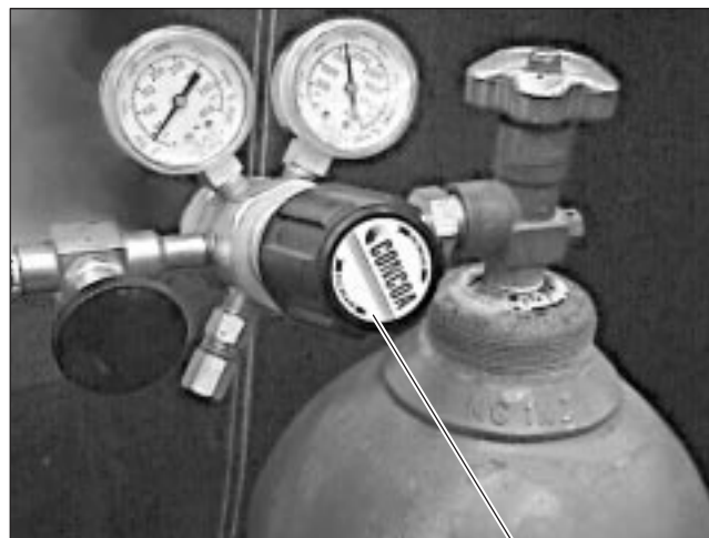
Multiple Gas Valve
