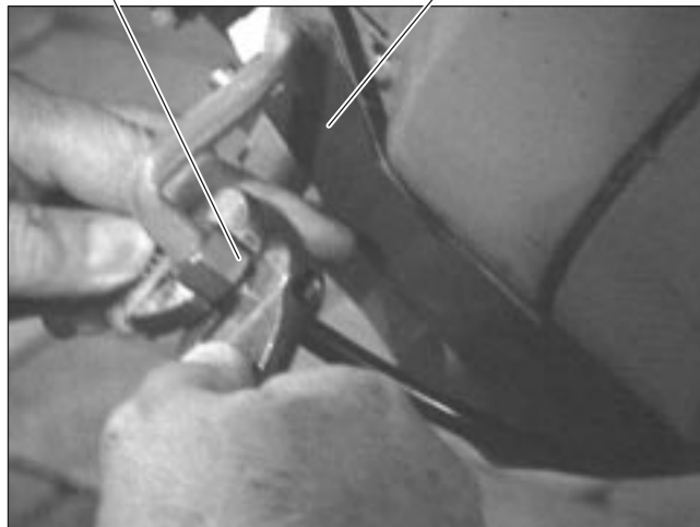
Air Line Reconnection
