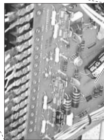
Power Supply Board
