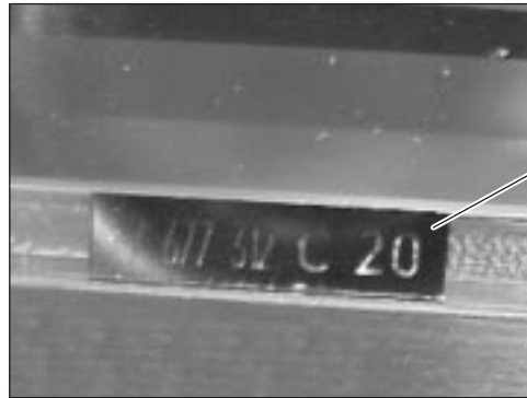
Read Head (Scanning Unit) Manufacturer's Number
