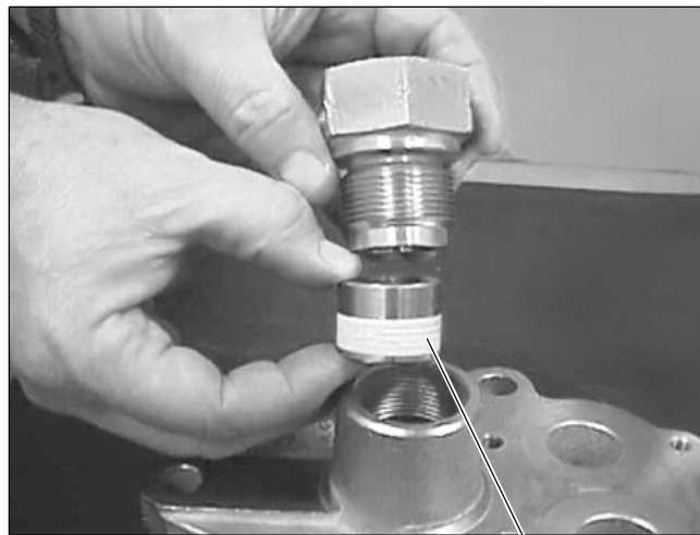
Male Gland, V-packing, and Female Gland
