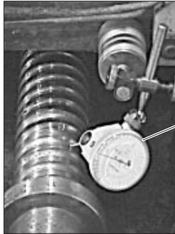
Indicator Set Up on Ball Screw Thread
