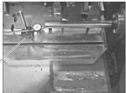
Indicator Set Up to Measure Lost Motion on Z-axis
