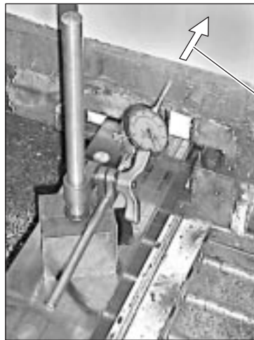
Increment Axis Five Times in the Positive Direction
