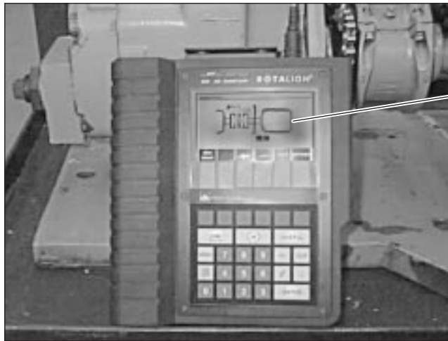
Aligned Shaft/Coupling Icon
