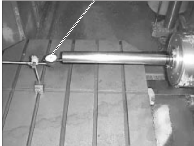
Dial Indicator Positioned to Measure Z-axis
