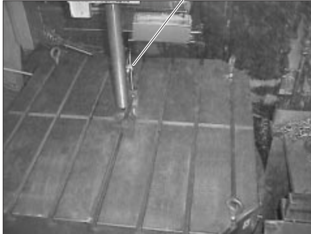
Indicator After Rotating Table 180°
