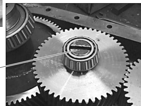
Slot in Transfer Assembly Shaft
